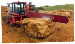
Revolutionary stone cutting machine which makes cutting the stone easier. (photo credit Ham & Doulting Stone)
